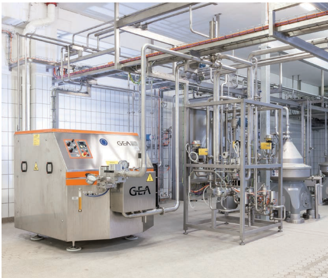
From left to right: the homogenizer by GEA Niro Soavi and the GEA Westfalia Separator Group respectively a Standomat MC, a skimming separator type MSI 140 and two bacteria removal separators type CSI 140 for extending shelf life.
