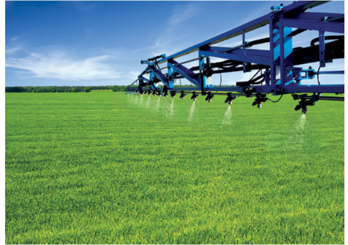
Figure 14: Nozzles with pulse width modulation in operation (source: TeeJet)
