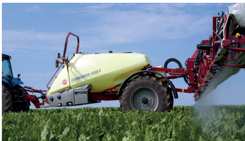
Figure 10: Spraying boom with air assistance, Hardi Twin Force system (source: Hardi)
