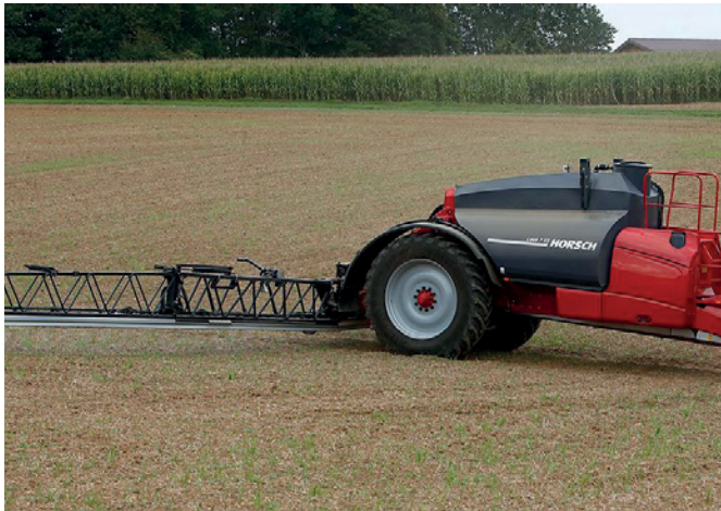
Figure 2: Stainless steel spray liquid tank (source: Horsch)
