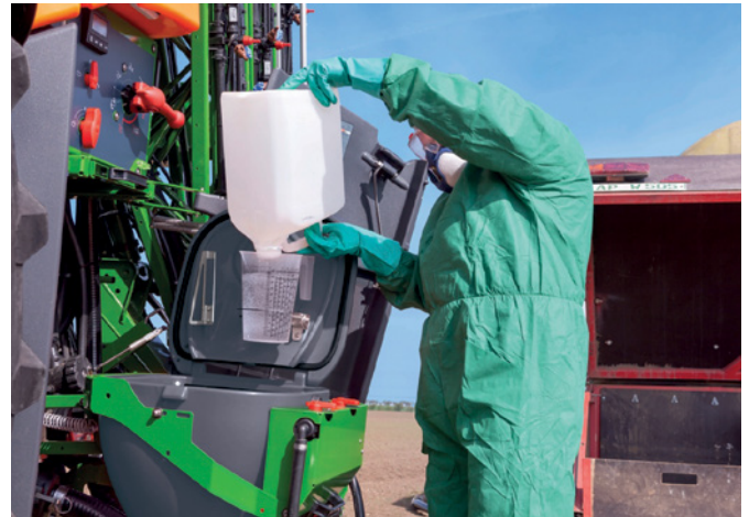
Figure 3: PE induction bowl (source: Amazone)
