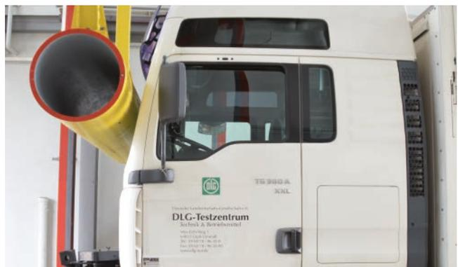
**ROPS tests on machines of up to 100 tonnes:** The DLG Test Center has two ROPS testing rigs that offer facilities for testing cabs on heavy-duty machinery with a max. weight up to 100 tonnes by applying forces of approx. 1,500kN horizontally and 2,000kN vertically.
