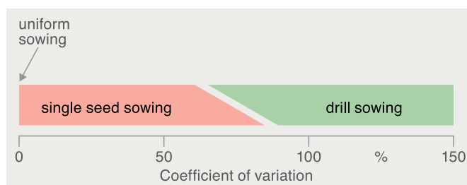
Figure 1: Coefficient of variation as an indicator of the uniformity of longitudinal distribution [Griepentrog, 1995 modified by Reckleben]
