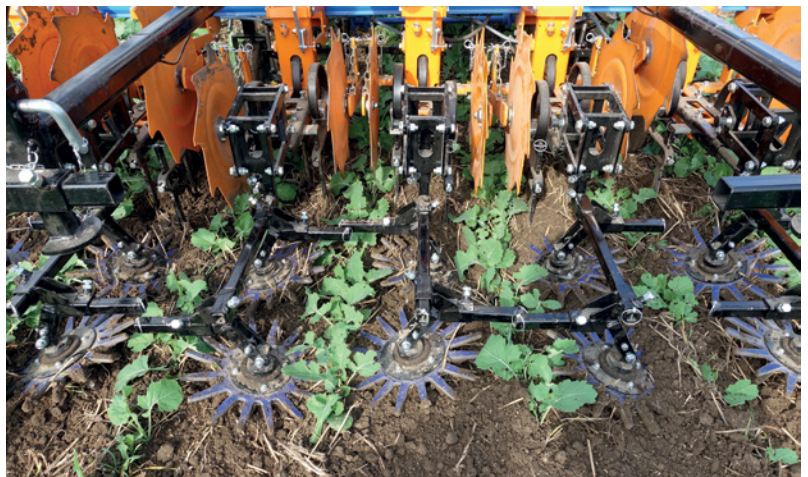
Figure 1: The Landwirtschaftskammer Niedersachsen is testing the use of finger hoes in trials in winter rape (source: Markus Mücke, Landwirtschaftskammer Niedersachsen)
