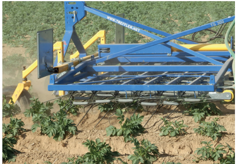
Figure 10: Tine harrows with indirect suspension are preferable on potato ridges, as they operate very consistently and are gentle on the crop (source: Markus Mücke, Landwirtschaftskammer Niedersachsen)
