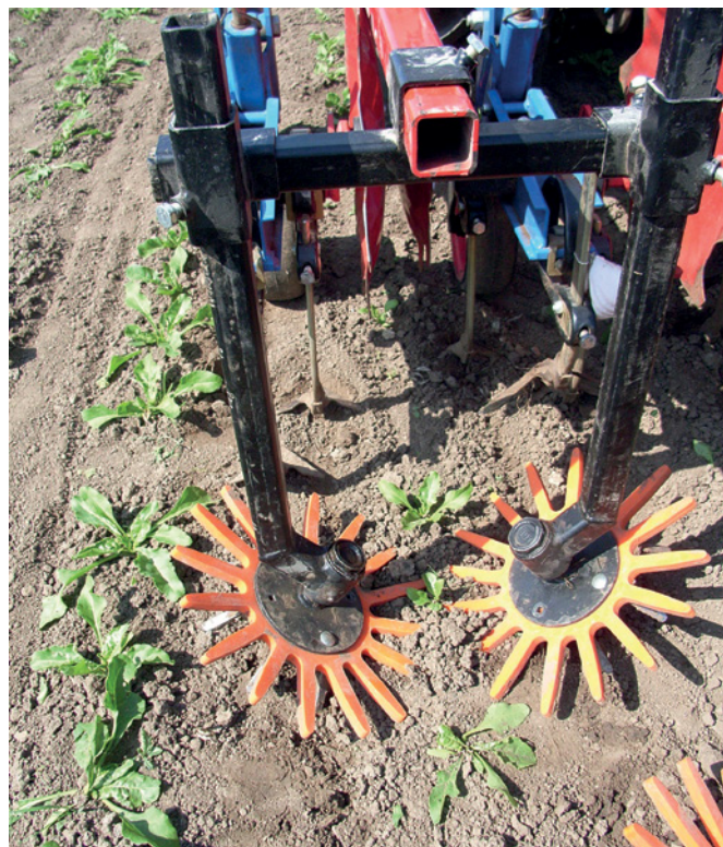
Figure 9: The finger hoes control weeds within the crop rows and can also be used for sugar beets (source: Markus Mücke, Landwirtschaftskammer Niedersachsen)
