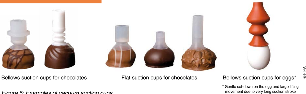
Figure 5: Examples of vacuum suction cups
