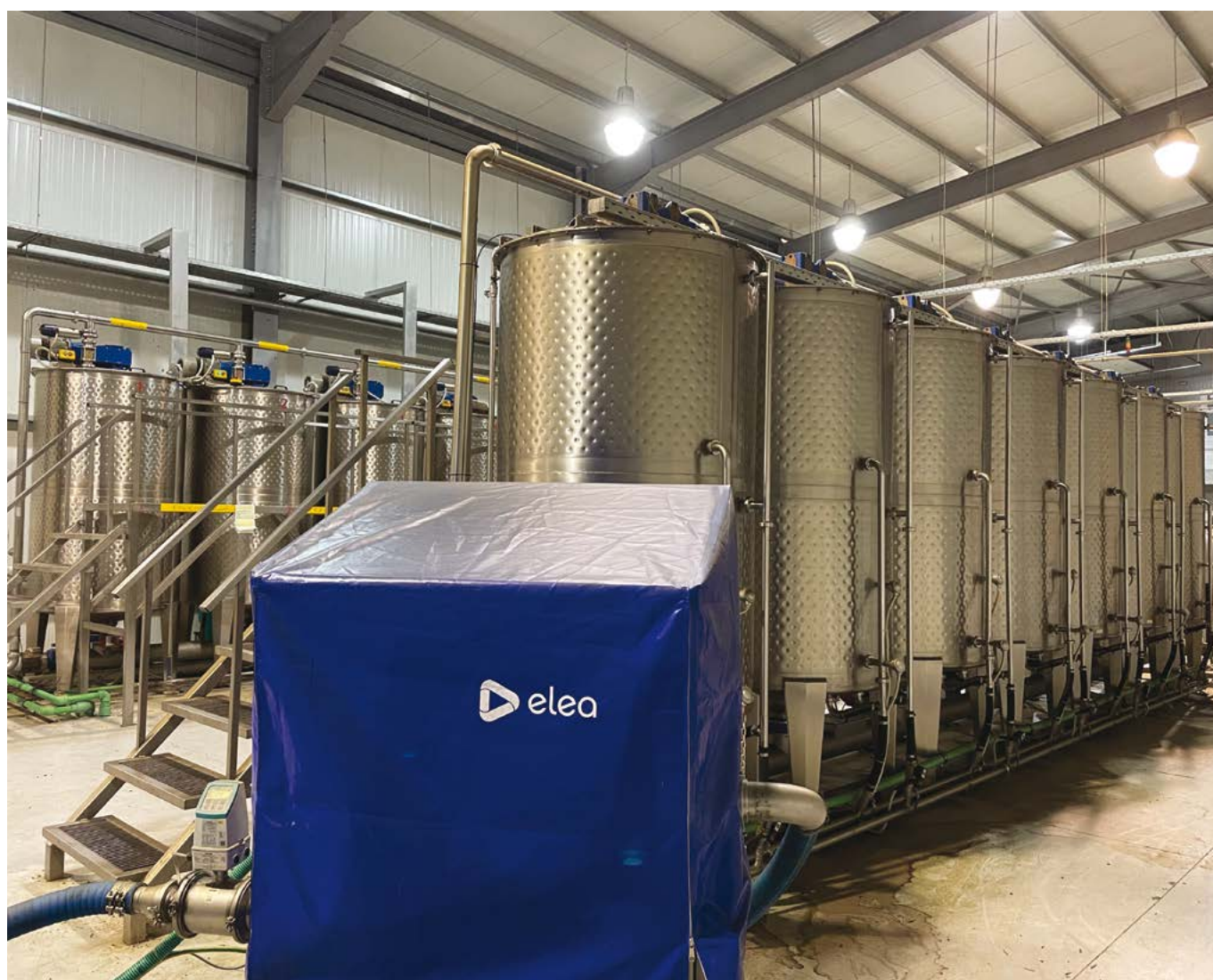
Figure 9: Industrial PEF unit installed in a Greek olive oil factory.
